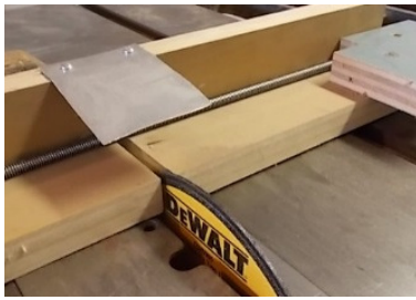
Figure 6. Jig for cutting rails and drive screws with abrasive disk on table saw. Note aluminum sheet for spark arresting on top and end stop for lengths.
