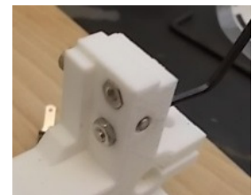
Figure 9. Nuts for limit switch are drawn into the syringe end holder.
