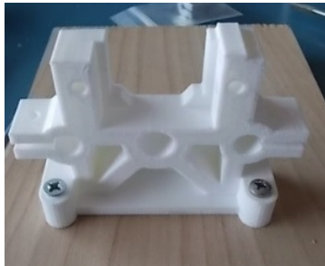
Figure 8. Syringe end holder screwed to plywood support.
