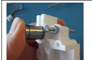
Figure 3. Inserting linear bearing into carriage assembly
