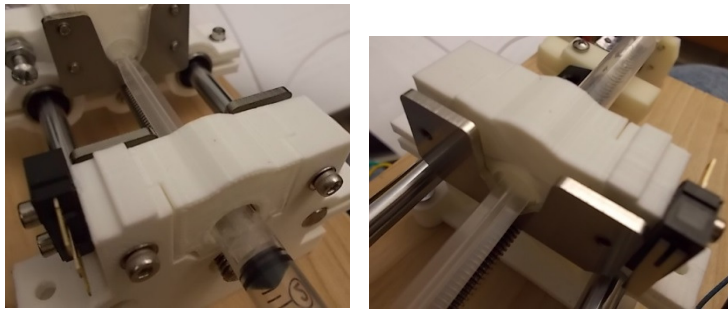
Figure 11. Syringe holder in mount held in place by syringe retaining plate.
